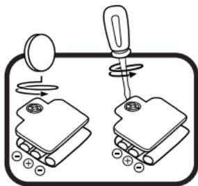
4. Install 3 new AAA (LR03/AM-4) batteries following the diagram inside the battery box. (For best performance, alkaline batteries or fully charged Ni-MH rechargeable batteries are recommended).
